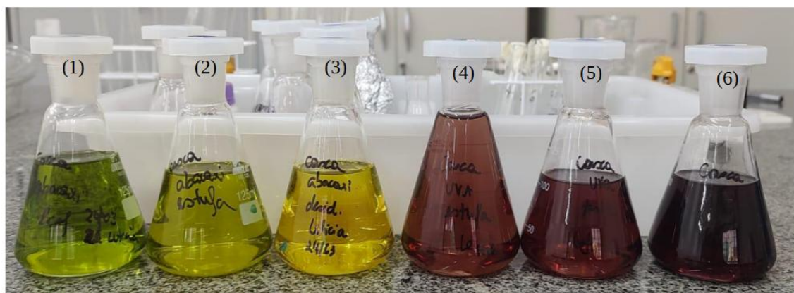
Figure 2: Alcoholic extract of pineapple peels dried by (1) Freeze dryer; (2) Oven with air circulation; (3) solar dehydrator and extract of grape peels dried by (4) Oven with air circulation; (5) Solar dehydrator; (6) Freeze dryer.
