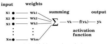
Figure 2 - Simplified diagram of an artificial neuron.
