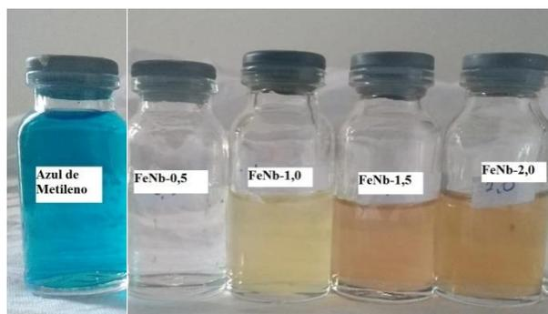
Figure 6. Pictures of the methylene blue removal system. From right to left: methylene blue solution, and solutions containing Fe / Nb solids in diets 0.1, 0.5, 1.0, 1.5 and 2.0, respectively.
