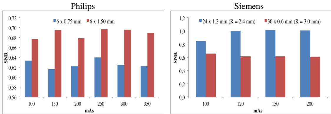
Figure 3: Influence of slice thickness on the signal to noise ratio with both scanners. For the Philips scanner, the slice thickness was equal to the reconstructed thickness; for the Siemens, the reconstructed slice thickness is slightly larger.
