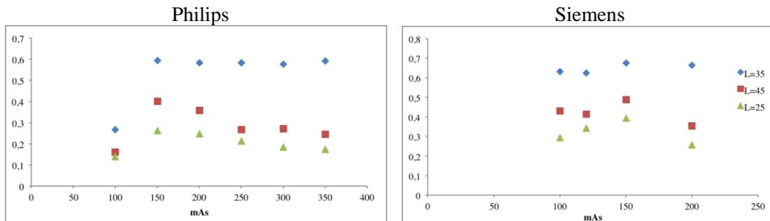
Figure 6: Image contrast vs. mAs with different visualizing window levels for both scanners.
