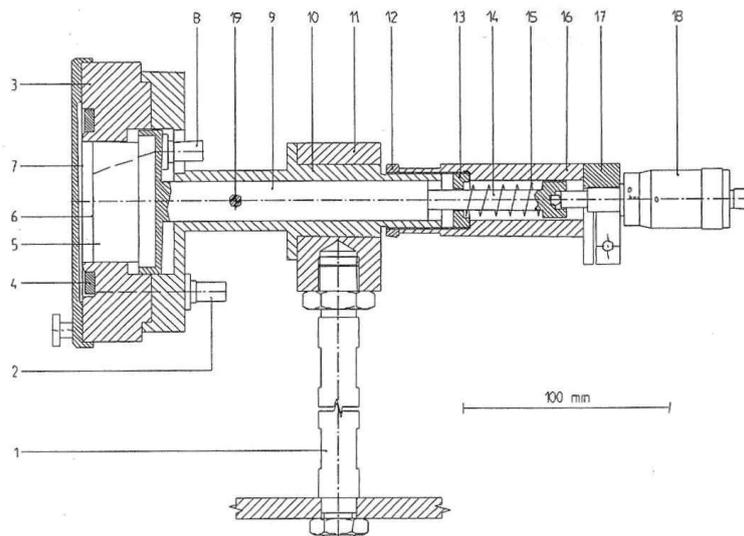
Figura 1: Cross section of the Böhm type extrapolation chamber. 1: stand, 2: polarizing voltage socket, 3: acrylic housing, 4: tension ring, 5: acrylic block, 6: graphite coated surface, divided into collecting electrode and guard ring, 7: entrance foil, 8: collecting electrode socket, 9: sliding-fit rod, 10: central guide for rod, 11: holder, 12: nut, 13: threaded ring, 14: bolt, 15: spring, 16: tube, 17: clamp, 18: micrometer screw, 19: pistonlocking screw.
