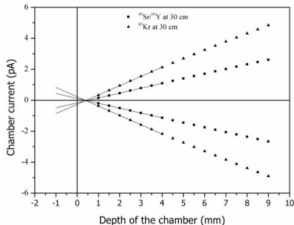
Figura 4: True null depth the 23392 PTW extrapolation chamber in the without filter  $^{90}\text{Sr}/^{90}\text{Y}$  and with filter  $^{85}\text{Kr}$  radiation beams.
