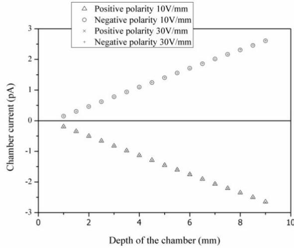
Figura 2: Response of the 23392 PTW extrapolation chamber for 10 and 30 V/mm with different depths and polarities in  $^{90}\text{Sr}+^{90}\text{Y}$  betaradiation beam.
